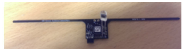
Figure 3: WISP 5 battery-free CRFID platform equipped with a photodiode
